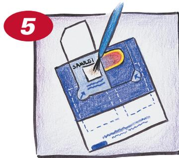
● Transfer the **WATER** sample by gently dabbing the bristles of the brush onto the small white square on the Test Card for about 5 seconds (some staining of the square may occur).
